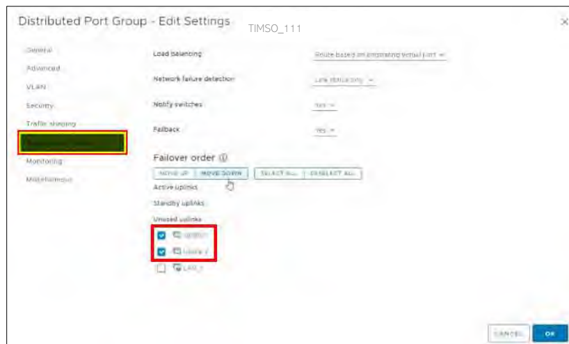
Figure 199. Move Uplink 1 and Uplink 2 to Unused Uplinks.
