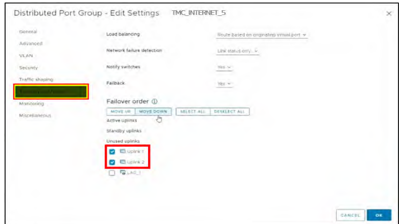
Figure 80. Move Uplink 1 and Uplink 2 to Unused Uplinks.
