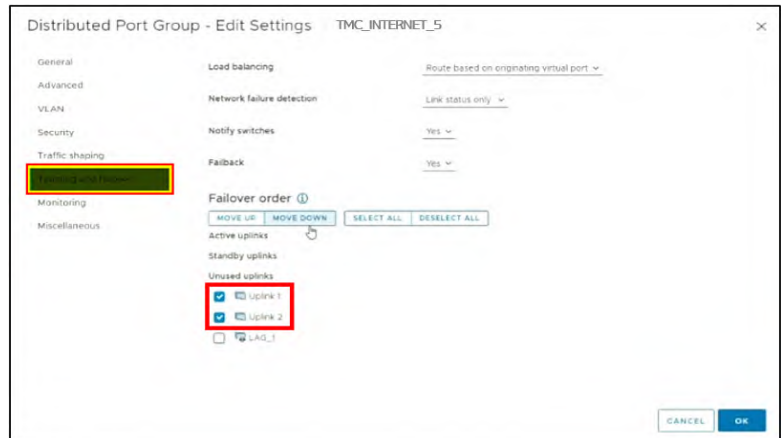
Figure 80. Move Uplink 1 and Uplink 2 to Unused Uplinks.
