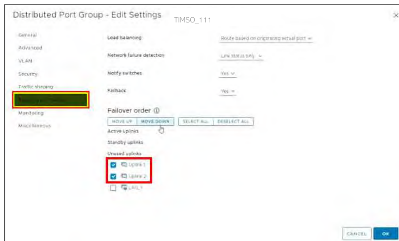
Figure 199. Move Uplink 1 and Uplink 2 to Unused Uplinks.
