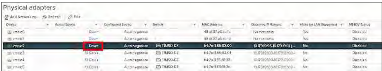
Figure 144. Confirm that the Port is Down
