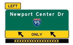
The signing on the southern two approaches to the Newport Center Dr roundabout shall include trailblazer signs for I-95 and Sawgrass Expressway. These approaches shall also include a roundabout guide sign with the legend for SW 10<sup>th</sup> Street as shown in the example below. The northern two approaches to the roundabout shall include a roundabout guide sign with no road name destinations.
