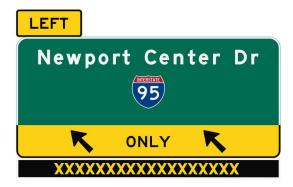
The signing on the southern two approaches to the Newport Center Dr roundabout shall include trailblazer signs for I-95 and Sawgrass Expressway. These approaches shall also include a roundabout guide sign with the legend for SW 10<sup>th</sup> Street as shown in the example below. The northern two approaches to the roundabout shall include a roundabout guide sign with no road name destinations.
