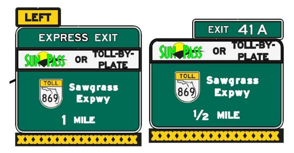
The destination on the guide signs from Sawgrass Expressway to the SW 10<sup>th</sup> Street Connector lanes shall include destinations for Newport Center Drive and the I-95 shield as shown below. The static sign width shall match the width of the lane status DMS.
