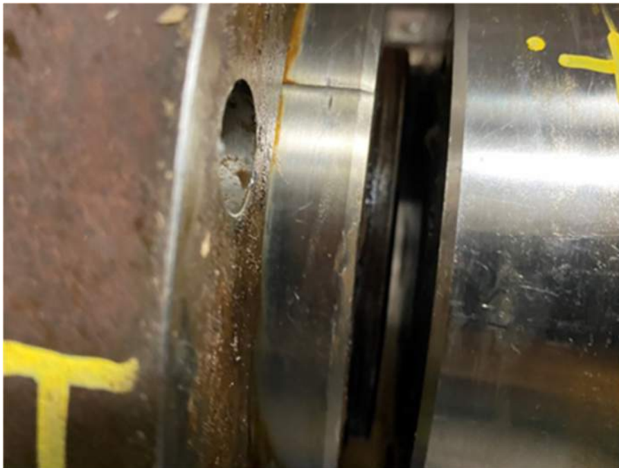
Photo 4: East coupling (bridge in closed position) - Note pinion shaft extending past hub face indicating movement of hub on shaft. Note "big" gap between the hubs
