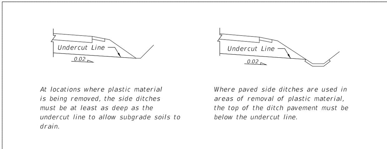
Tabulate subsoil excavation areas and volumes on the right side of the cross section sheets. The fill quantities (areas and volumes) must include areas and volumes required to fill the excavated areas created by subsoil removal. See example given in **Section 3.1** of this chapter.
