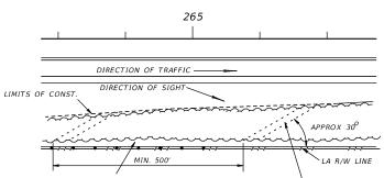
10' STRIP WHICH MAY BE CLEARED FOR FENCE CONSTRUCTION WITH SELECTED DESIRABLE TREES ALLOWED TO REMAIN, AS DIRECTED BY THE ENGINEER.
