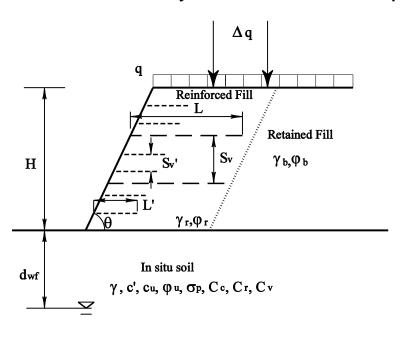
**Exhibit 31-A Geosynthetic Reinforced Soil Slopes**
