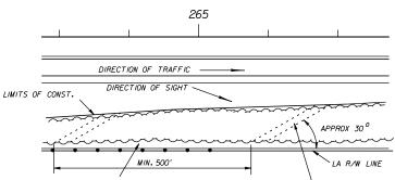
IO'STRIP WHICH MAY BE CLEARED FOR FENCE CONSTRUCTION WITH SELECTED DESIRABLE TREES ALLOWED TO REMAIN, AS DIRECTED BY THE ENGINEER.
