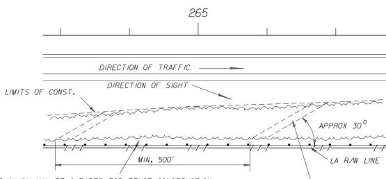
IO' STRIP WHICH MAY BE CLEARED FOR FENCE CONSTRUCTION WITH SELECTED DESIRABLE TREES ALLOWED TO REMAIN, AS DIRECTED BY THE ENGINEER.
