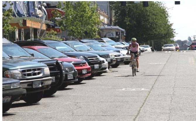
14 15 Back in Angle Parking, Seattle, WA 16 (Source: Photo - Dan Burden) 17
