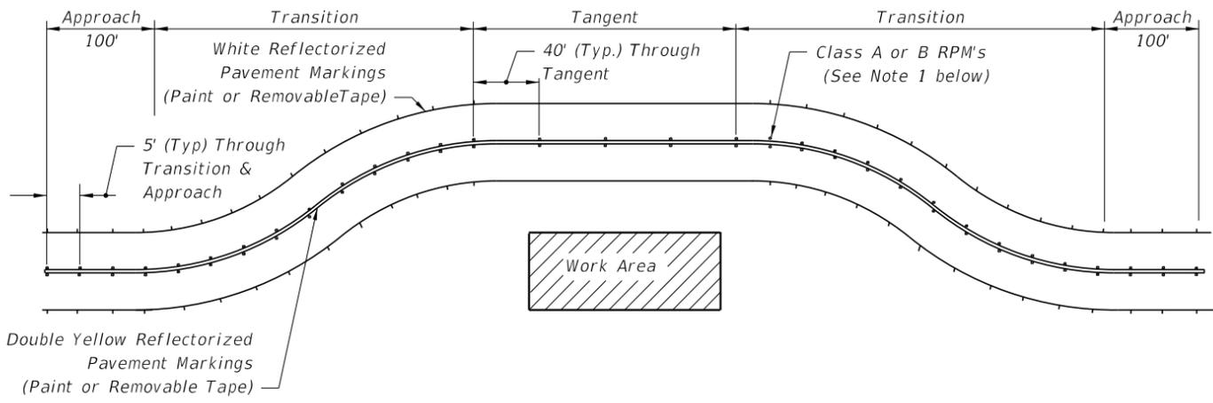
**USE OF RPM'S TO SUPPLEMENT PAINT OR REMOVABLE TAPE IN WORK ZONES**
