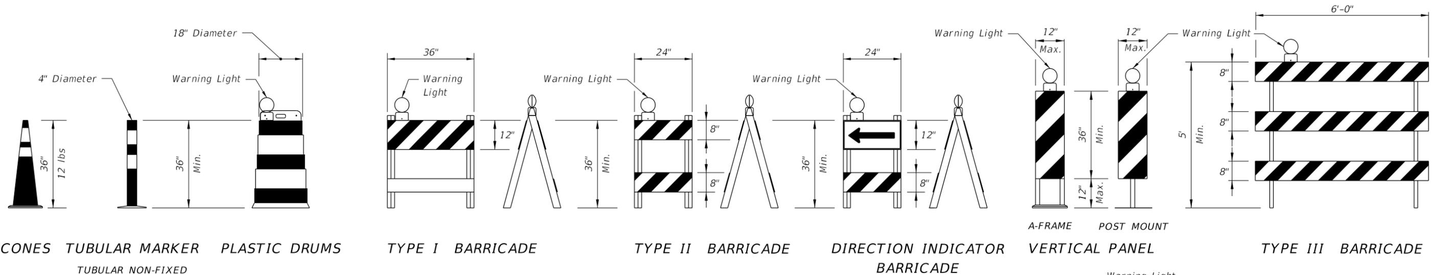
TUBULAR NON-FIXED MARKER TO BE USED DURING DAYLIGHT ONLY
