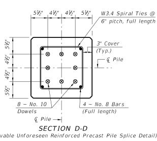
(See Nondrivable Unforeseen Reinforced Precast Pile Splice Detail)
