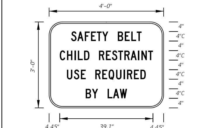
FTP-45-06 4' X 3' 5" Radii 3/4" Border 4" Series C Legend White Background Black Legend and Border
