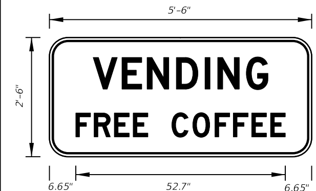
FTP-74-06 5'-6" X 2'-6" 4" Radii 3/4" Border 6" Series D Legend Blue Background White Legend and Border
