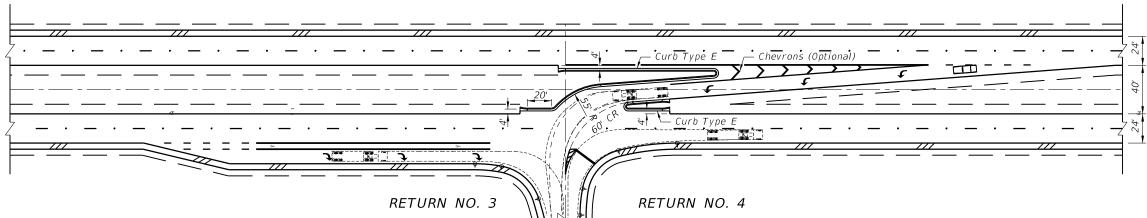
NOTE: Return configurations for each quadrant must be analyzed independently to assure adequate return pavement for semi-trailer inside tracking. The depicted design only applies where roads and streets intersect at 90° to the mainline. Swept paths are by AutoTURN 4.0 for the AASHTO 2001 SU and WB-40 tractor-semitrailer.
