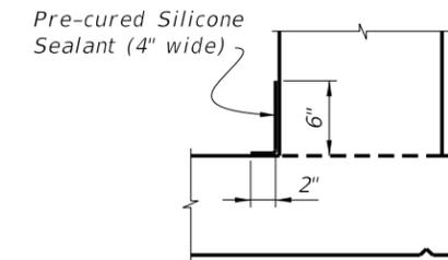
DETAIL "A" - SECTION AT INTERMEDIATE OPEN JOINT
