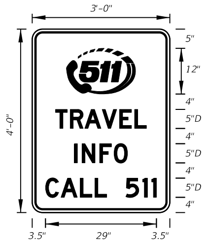
FTP-67-06 3' X 4' 2" Radii 3/4" Border 5" Series D Legend Blue Background White Legend and Border
