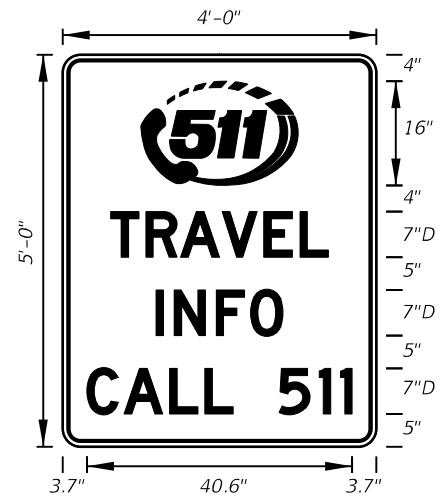
FTP-66-06 4' X 5' 2" Radii 3/4" Border 7" Series D Legend Blue Background White Legend and Border
