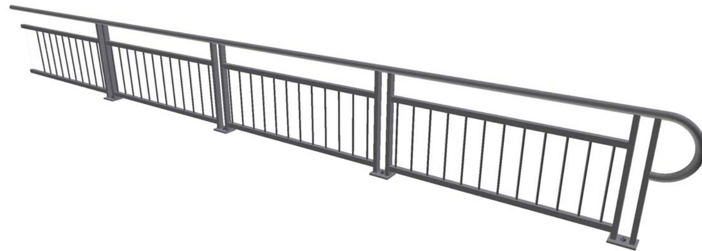
3D VIEW OF RAILING WITH TYPE 1 - PICKET INFILL PANEL (42" Height shown, 54" Height Similar)
