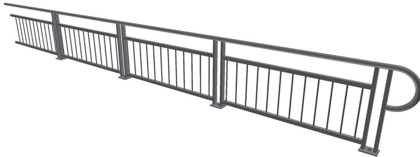
3D VIEW OF RAILING WITH TYPE 1 - PICKET INFILL PANEL (42" Height shown, 54" Height Similar)
