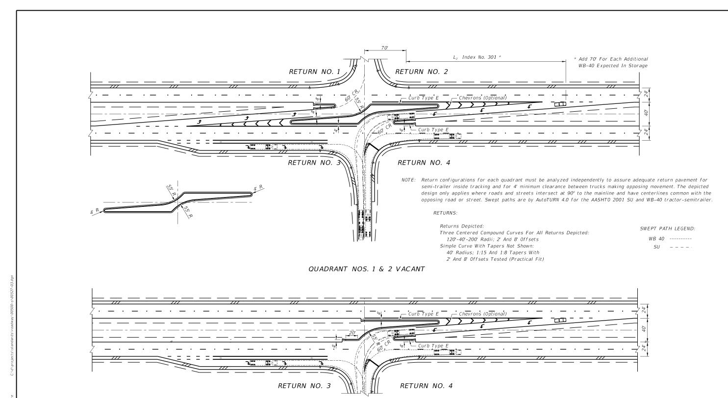
NOTE: Return configurations for each quadrant must be analyzed independently to assure adequate return pavement for semi-trailer inside tracking. The depicted design only applies where roads and streets intersect at 90° to the mainline. Swept paths are by AutoTURN 4.0 for the AASHTO 2001 SU and WB-40 tractor-semitrailer.
