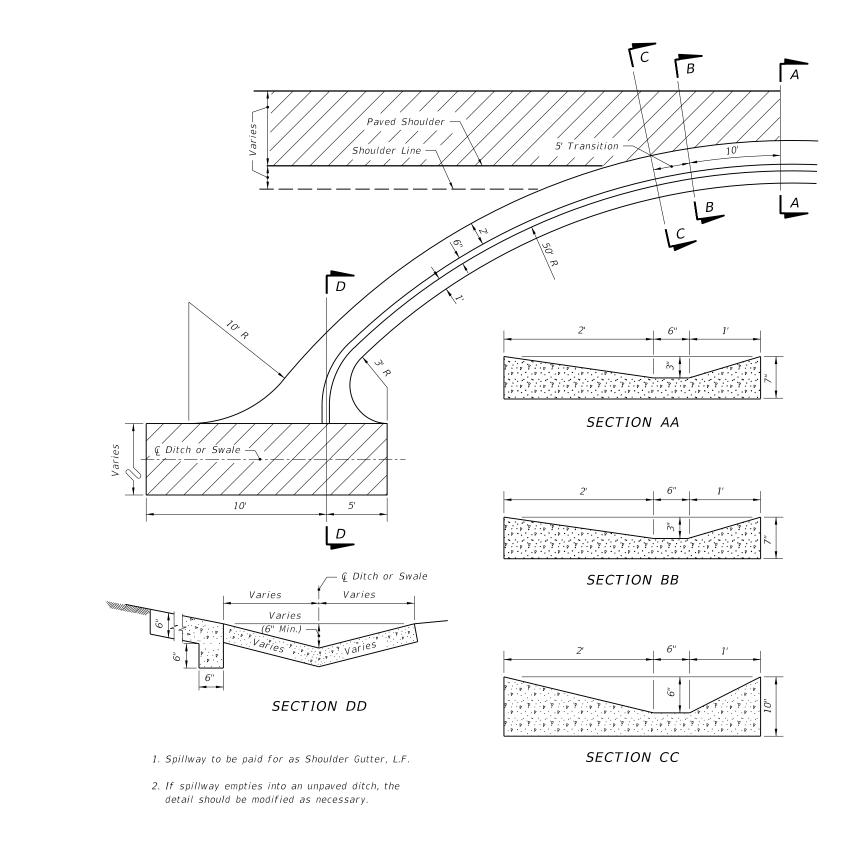
DETAIL OF CONCRETE SPILLWAY AT END OF SHOULDER GUTTER (TO BE USED WHERE INLETS, PIPES & ENDWALLS ARE IMPRACTICAL)
