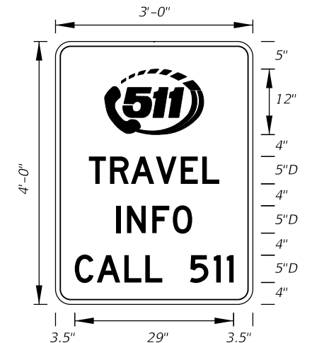
FTP-67-06 3' X 4' 2" Radii 3/4" Border 5" Series D Legend Blue Background White Legend and Border
