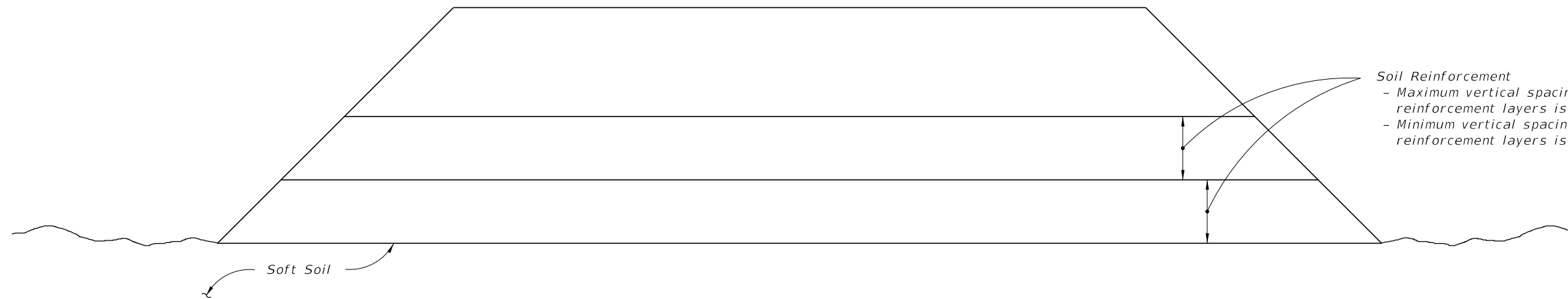
GEOSYNTHETIC REINFORCED FOUNDATIONS CONSTRUCTED ON SOFT SOILS
