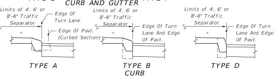
For Curb And Curb & Gutter Types, See Index No. 300 \* Option I Separators Shown (Refer To Index No. 302)
