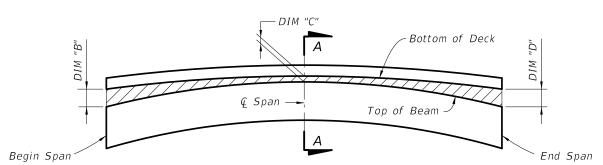
BUILD-UP DIAGRAM FOR CREST VERTICAL CURVE SPANS
