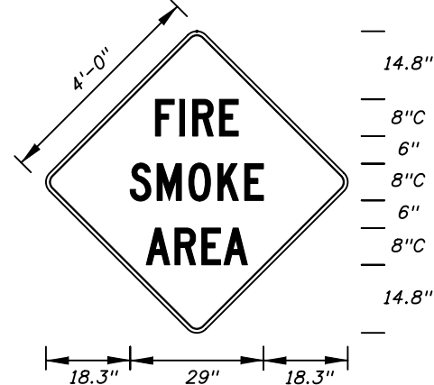
FTP-71-06 4' X 4' 2" Radii 3/4" Border 8" Series C Legend Yellow Background Black Legend and Border
