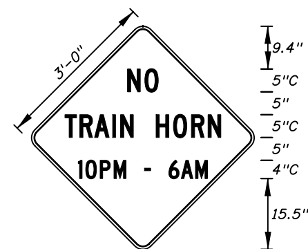
FTP-62-06 3' X 3' 2" Radii \frac{3}{4} " Border 4" and 5" Series C Legend Yellow Background Black Legend and Border
