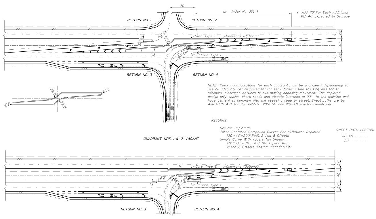
NOTE: Return configurations for each quadrant must be analyzed independently to assure adequate return pavement for semi-trailer inside tracking. The depicted design only applies where roads and streets intersect at 90° to the mainline. Swept paths are by AutoTURN 4.0 for the AASHTO 2001 SU and WB-40 tractor-semitrailer.
