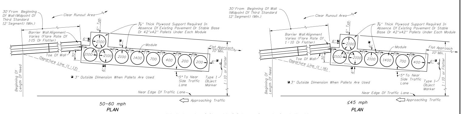
Note: Numbers shown inside modules indicate mass in pounds of sand. All modules are approximately 3' in diameter with heights ranging from 3' to 3'-9".
