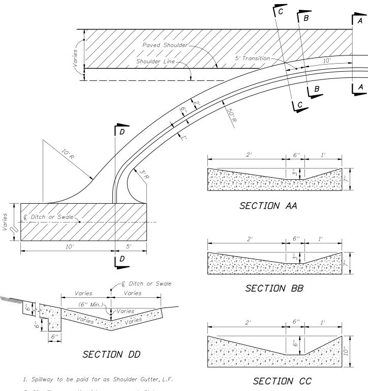
2. If spillway empties into an unpaved ditch, the detail should be modified as necessary.
