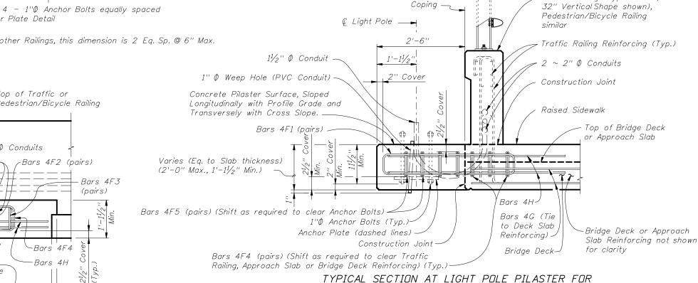
TYPICAL SECTION AT LIGHT POLE PILASTER FOR APPROACH SLAB OR BRIDGE DECK THICKNESS 1'-11/2" OR GREATER
