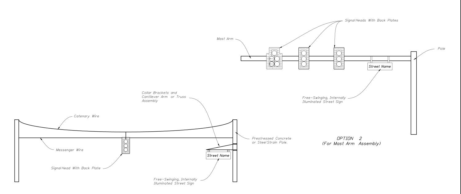
OPTION 1 (For Span Wire Assembly)
