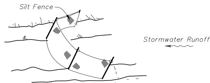
Silt Fence Protection In Ditches With Intermittent Flow
