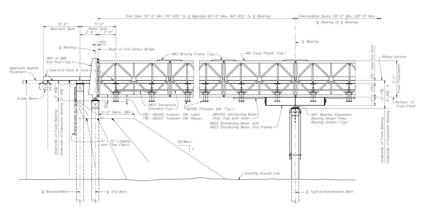
ELEVATION VIEW (TIMBER PILES SHOWN, STEEL H PILES AND STEEL PIPE PILES SIMILAR)
