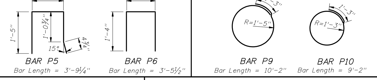
BAR P5 Bar Length = 3'-9 1/4" BAR P6 Bar Length = 3'-5 1/2" BAR P9 Bar Length = 10'-2" BAR P10 Bar Length = 9'-2"
