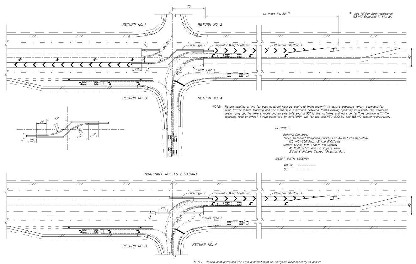
NOTE: Return configurations for each quadrant must be analyzed independently to assure adequate return pavement for semi-trailer inside tracking. The depicted design only applies where roads and streets intersect at 90° to the mainline. Swept paths are by AutoTURN 4.0 for the AASHTO 200ISU and WB-40 tractor-semitrailer.
