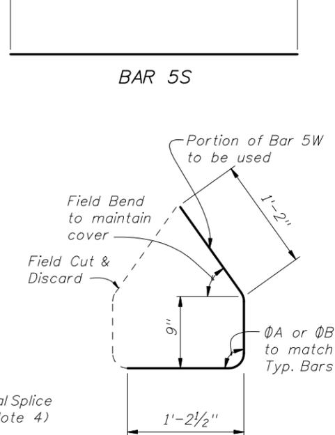
TRANSITION STIRRUP BAR 5W To Be Field Cut and Bent (10 required per Railing End Transition)
