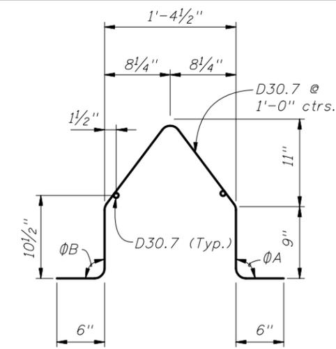
Welded Wire Reinforcement (WWR) Piece No. 1
