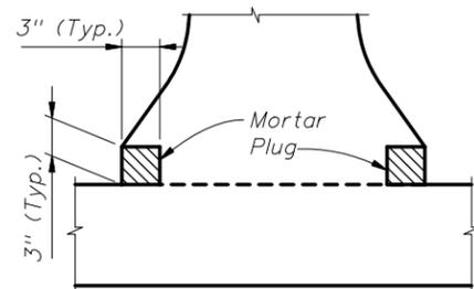
DETAIL "B" - SECTION AT INTERMEDIATE OPEN JOINT
