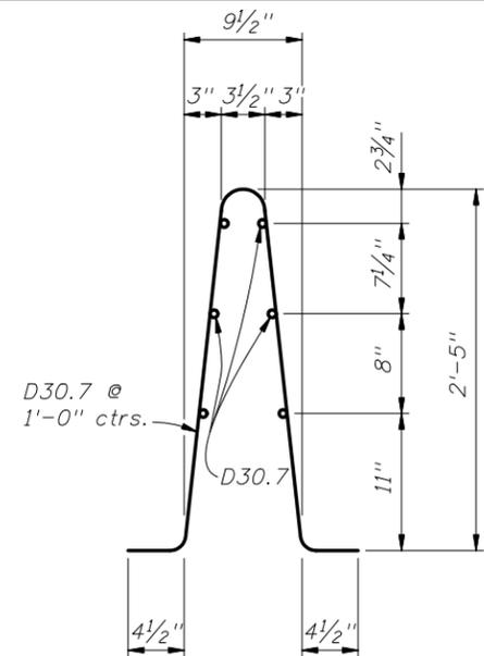
Welded Wire Reinforcement (WWR) Piece No. 2
