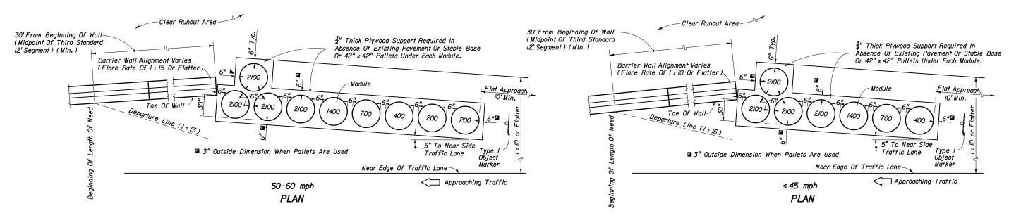
Note: Numbers shown inside modules indicate mass in pounds of sand. All modules are approximately 3' in diameter with heights ranging from 3' to 3'-9".
