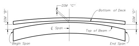
BUILD-UP DIAGRAM FOR CREST VERTICAL CURVE SPANS
