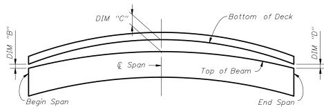
BUILD-UP DIAGRAM FOR CREST VERTICAL CURVE SPANS
