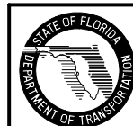
FTP-62-06 3' X 3' 2" Radii 3/4" Border 4" and 5" Series C Legend Yellow Background Black Legend and Border
