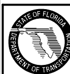
FTP-51-06 3' X 2' 3" Radii 3/4" Border 4" Series E Legend White Background Black Legend and Border
