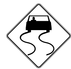
W8-5 SLIPPERY WHEN WET SIGN See Note 11.
