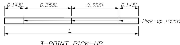
PILE PICK-UP DETAILS
