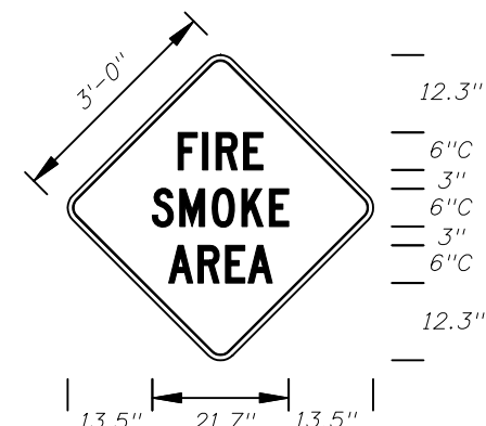
FTP-72-06 3' X 3' 2" Radii 3/4" Border 6" Series C Legend Yellow Background Black Legend and Border
