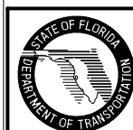
FTP-29-06 2'-0" X 1'-0" 2" Radii \frac{5}{8} " Border 4" Series C Legend Yellow Background Black Legend and Border
