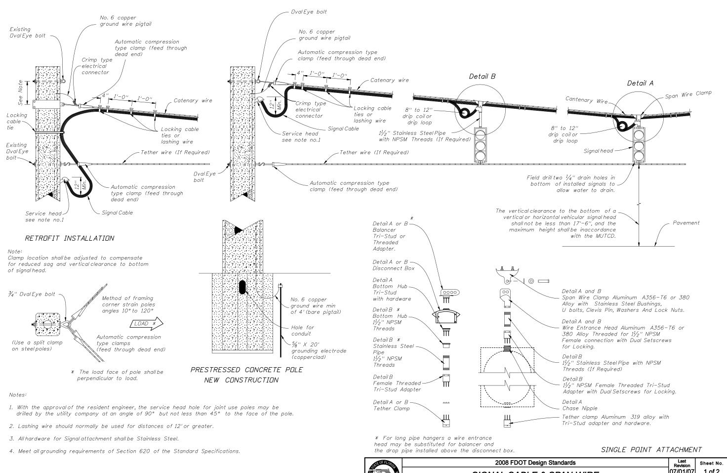
SIGNAL CABLE & SPAN WIRE INSTALLATION DETAILS
