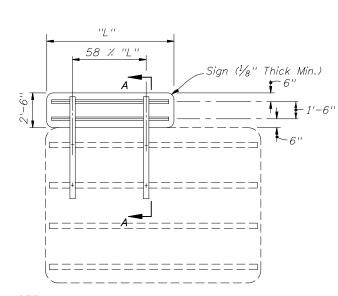
NOTE: Exit numbering panel shall be located to the right side for right exit and to the left for left exit.
