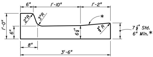
\* When used on high side of roadways, the cross slope of the gutter shall match the cross slope of the adjacent pavement. The thickness of the lip shall be 6", unless otherwise shown on plans.
