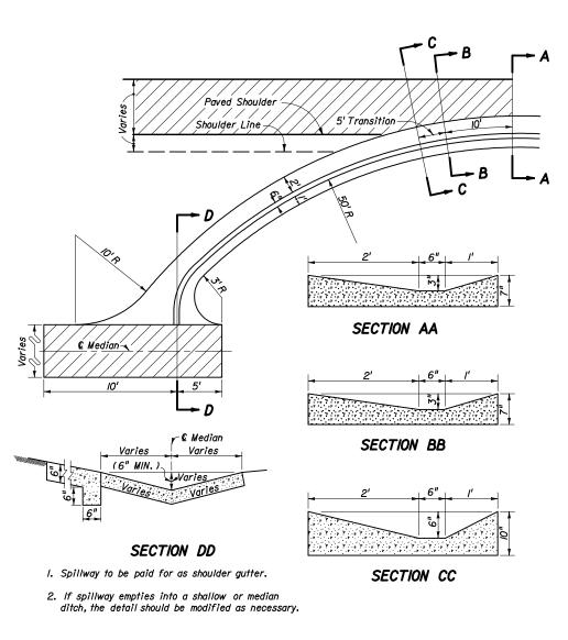
**DETAIL OF CONCRETE SPILLWAY AT END OF SHOULDER GUTTER** (TO BE USED WHERE INLETS, PIPES & ENDWALLS ARE IMPRACTICAL)
