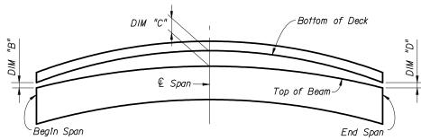
BUILD-UP DIAGRAM FOR CREST VERTICAL CURVE SPANS - CONTROL AT BEGIN OR END SPAN (ALONG € BEAM) (CASE 4)
