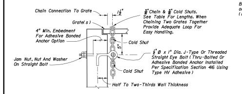
NOTE: When Alternate G grate is specified, the chain, bolt, nuts, washer and cold shuts shall be galvanized in accordance with the specifications for the grate.
