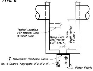
NOTE: Sump bottom appropriate for all manhole and inlet types. Sumps are to be constructed in inlet and manholes connected to French Drains unless excluded in the plans. At other locations, sump is to be constructed only where called for in the plans. Weep holes to be constructed in sump bottom only where called for in the plans. Cost of sump bottom and weep hole to be included in the contract unit price for inlet or manhole.
