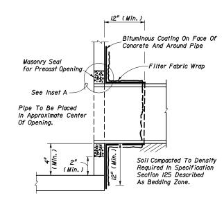
FILTER FABRIC WRAP ON GROUTED PIPE TO STRUCTURE JOINT
