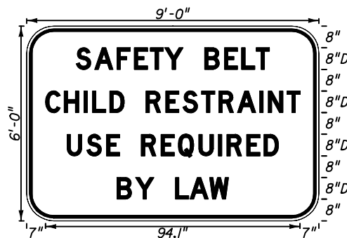
FTP-44-04 9' X 6' 9" Radii 3/4" Border 8" Series D Legend White Background Black Legend & Border
