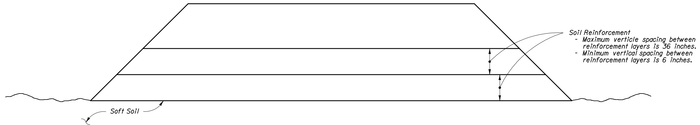
GEOSYNTHETIC REINFORCED FOUNDATIONS CONSTRUCTED ON SOFT SOILS
