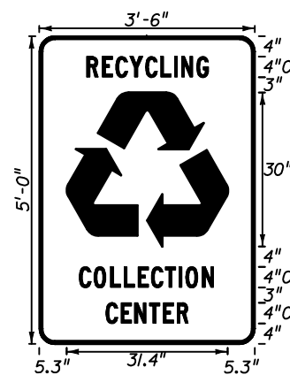
FTP-48-04 3'-6" X 5' 3" Radii 4" Series C Legend Green Background White Legend, Border & Symbol
