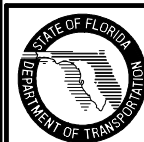
FTP-39-04 Freeway Sign 4' X 4' 3" Radii 3/4" Border 6" Series D White Background Black Legend & Border
