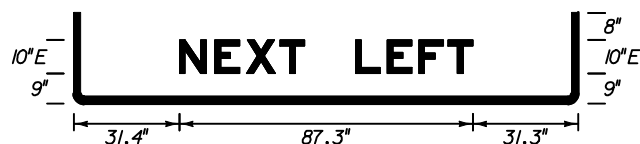
FTP-7B-04 12'-6" X 7' 3" Radii 2" Border Series E Legend Green Background White Legend & Border
