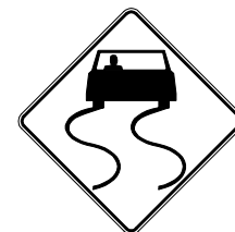
W8-5 SLIPPERY WHEN WET SIGN See Note 11.
