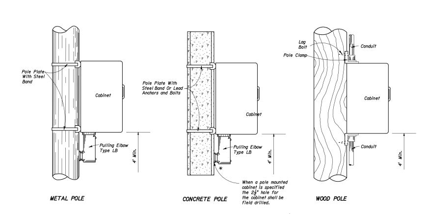
Liquid tight flexible conduit is approved for use from the electrical disconnect to the cabinet when both are installed on the same pole.
