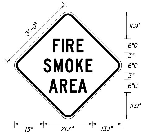
FTP-73-06 3' X 3' Series C Legend 2" Radii 3/4" Border Yellow Background Black Legend & Border
