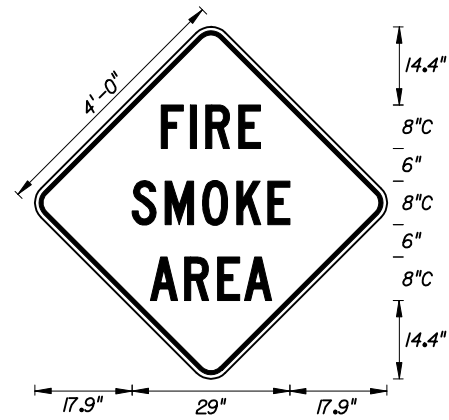
FTP-72-06 4' X 4' Series C Legend 3" Radii 3/4" Border Yellow Background Black Legend & Border
