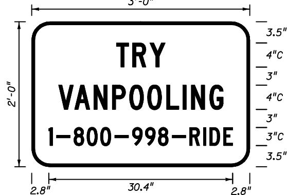
FTP-58-04 3' X 2' 3" Radii 4" Series C Legend 3" Series C Legend Blue Background White Legend & Border
