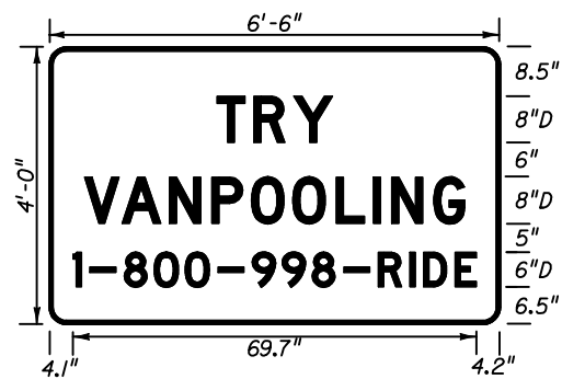
FTP-57-04 6'-6" X 4' 3" Radii 8" Series D Legend 6" Series D Legend Blue Background White Legend & Border
