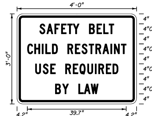
FTP-45-04 4' X 3' 1 1/2" Radii 3/4" Border 4" Series C Legend White Background Black Legend & Border
