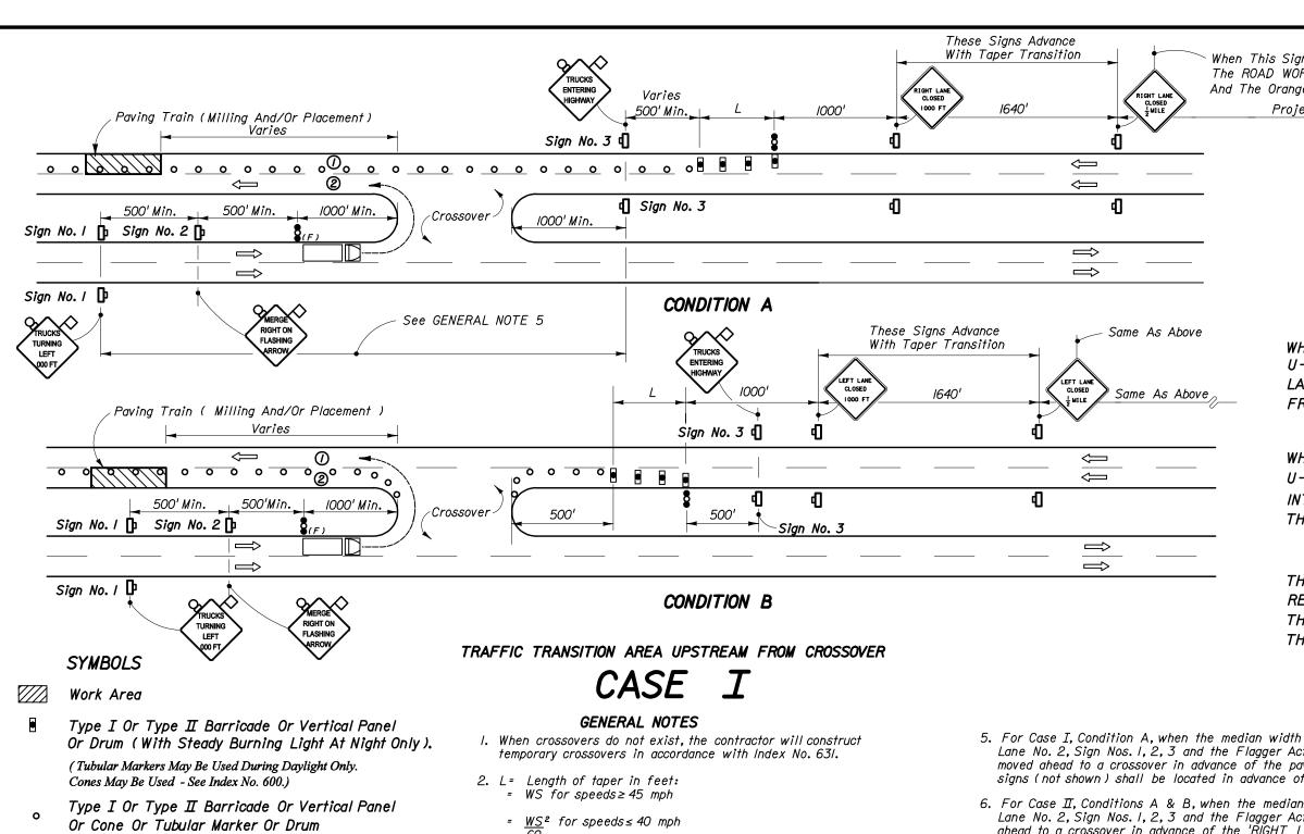
When This Sign Conflicts With ROAD WORK & MILE Sign, The ROAD WORK & MILE Sign Shall Be Temporarily Removed And The Orange Flag And Type B Light Attached To This Sign. Project Advance Warning Signing
