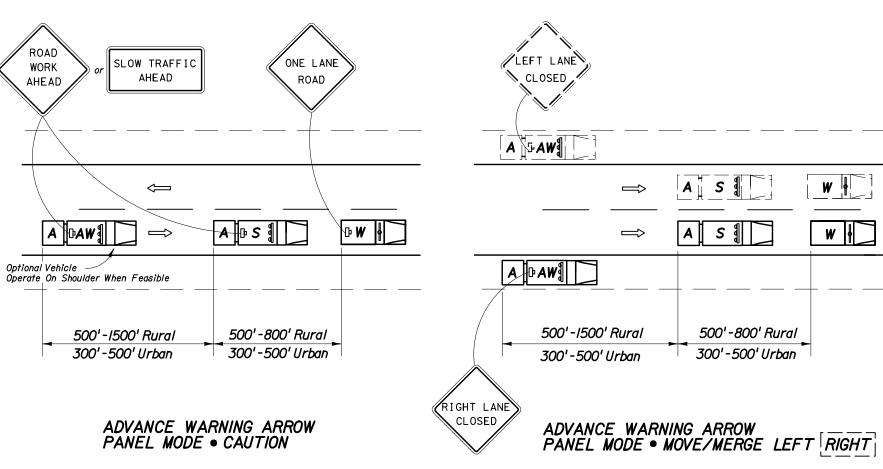
I. Shadow and Advance Warning Vehicle shall display rotating/strobe lights.
